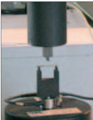
Dynamometer with accessory for carrying out the Schwickerath crack initiation test: a new method used to determine quantitatively the metal-ceramic bond strength.
